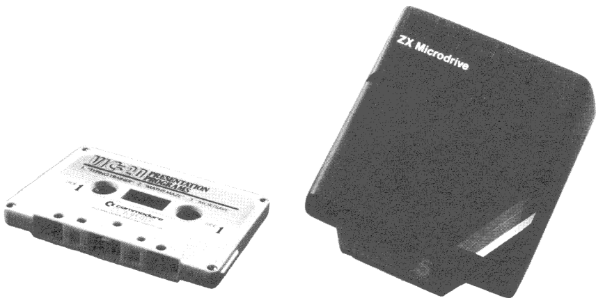
Figure 1.4 A cassette and a microdrive.
